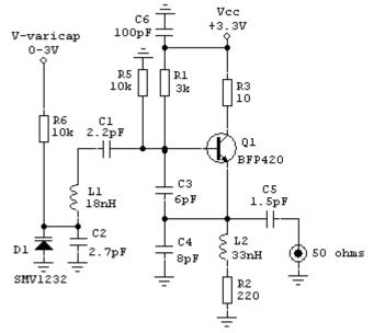
1GHz - 1.2GHz series tuned Colpitts VCO (Clapp VCO)
