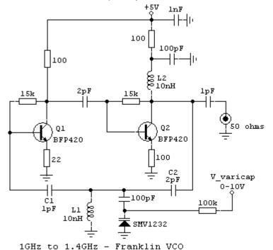
In this circuit, each stage shifts phase 180° so that the total phase shift is 360° which is equivalent to zero phase shift. We may say that one stage serves as the phase inverting element in place of the RC or LC network which generally performs this function. It is, from an analytical viewpoint, immaterial which stage we choose to look upon as amplifier or phase inverter.
