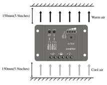
Figure 3-1 Mounting and cooling
